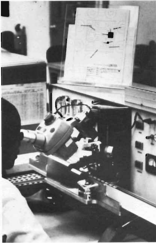
Figure 4. FETRON Production. Methods used for assembly are the best industry quality control standards, MIL-STD-883. Assembly procedures are carefully planned and carried out under ultra-clean conditions to maximize FETRON reliability.
