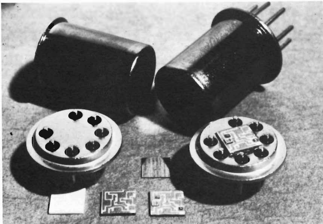
Figure 5. FETRON Assembly Steps. The FETRON thick film circuit is shown (1) as a clean substrate, (2) with conductive film, (3) with circuit etched, and (4) with circuit chips attached. The completed circuit is then soldered to the header and connected to the posts with gold wires. The header is then hermetically sealed with a nickel-plated cap.
