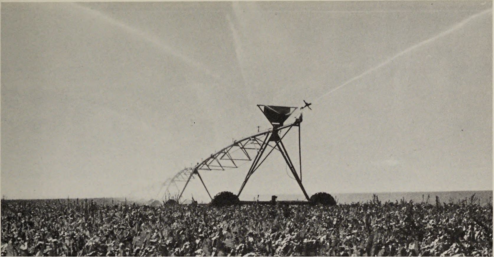
A pivot sprinkler system on a developed Desert Land Entry in southwest Idaho. The pivot turns to make a complete circle. Most pivots can irrigate about 140 acres. Sprinklers are placed along the entire length of the pivot arm.
