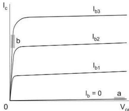
**FIG. 2.3** Transistor characteristics showing high-resistance (cut-off) region Oa and low-resistance (saturation) region Ob. Typical ‘off’ and ‘on’ operating states are shown by the shaded areas a and b respectively.
