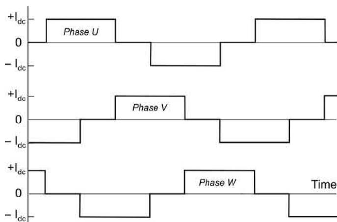
FIG. 9.25 Idealised steady state motor phase current waveforms.
