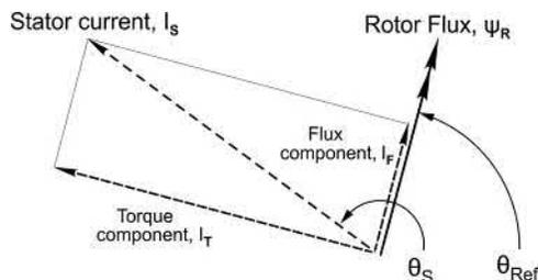
**FIG. 8.18** Stator current and rotor flux reference angles.
