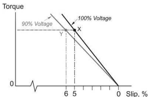
FIG. 6.15 Influence of stator supply voltage on torque-speed curves.
