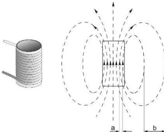
**FIG. 1.7** Multi-turn cylindrical coil and pattern of magnetic flux produced by current in the coil. (For the sake of clarity, only the outline of the coil is shown on the right.)
