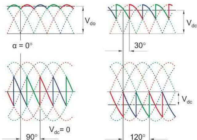
FIG. 2.13 Output voltage waveforms for three-phase fully-controlled thyristor converter supplying an inductive (motor) load, for various firing angles from  $0^\circ$  to  $120^\circ$ . The mean d.c. voltage is shown by the horizontal line, except for  $\alpha = 90^\circ$  where the mean d.c. voltage is zero.
