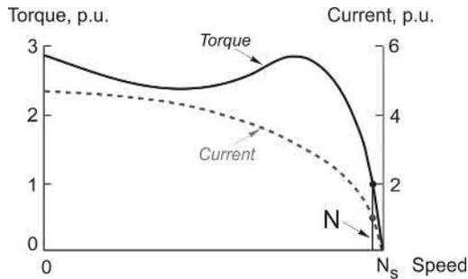
**FIG. 6.13** Typical torque-speed and current-speed curves for a general-purpose industrial double cage motor.
