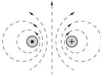
**FIG. 1.6** Magnetic flux lines produced by current in a parallel go and return circuit.
