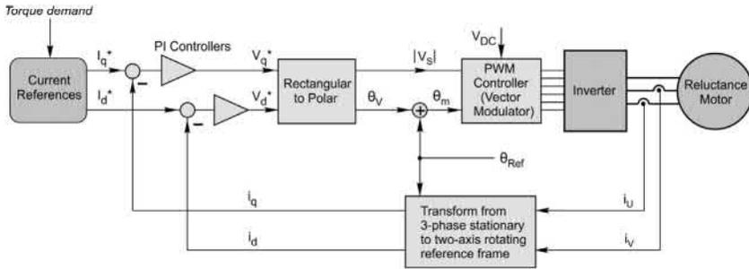
FIG. 9.31 Field oriented control scheme for reluctance motor.
