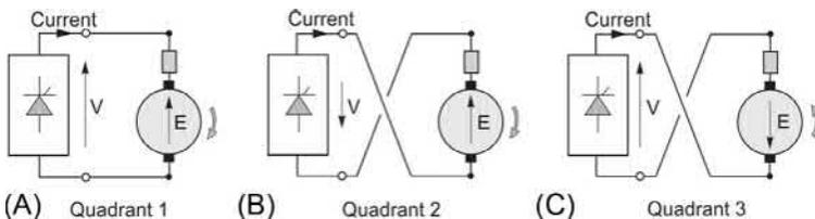
**FIG. 4.8** Stages in motor reversal using a single-converter drive and mechanical reversing switch.
