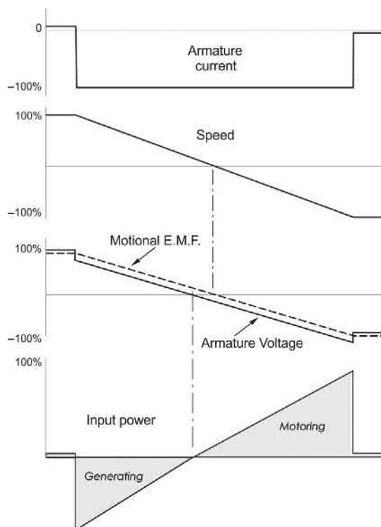
**FIG. 3.13** Regenerative reversal of d.c. motor from full-speed forward to full-speed reverse, at maximum allowable torque (current).
