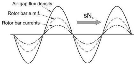
**FIG. 5.17** Pattern of air-gap flux density, induced e.m.f. and current in cage rotor bars at low values of slip.
