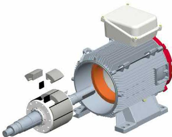
**FIG. 9.34** Permanent magnet synchronous machine in a standard IEC frame. (Courtesy Nidec—Leroy Somer.)
