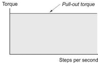
**FIG. 10.14** Steady-state operating region with ideal constant-current drive. (In such idealised circumstances there would be no limit to the stepping rate, but as shown in Fig. 10.18, a real drive circuit imposes an upper limit.)
