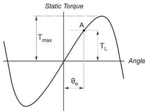
FIG. 10.10 Static torque–angle curve showing step position error ( $\theta_e$ ) resulting from load torque  $T_L$ .
