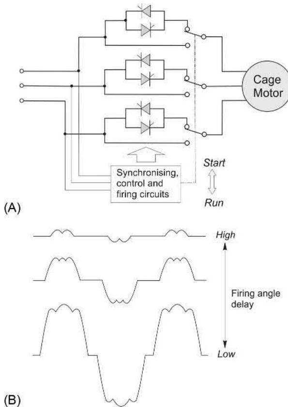
**FIG. 6.4** (A) Thyristor soft-starter, (B) typical motor current waveforms.
