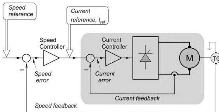
**FIG. 4.12** Schematic diagram of analogue controlled-speed drive with current and speed feedback control loops.
