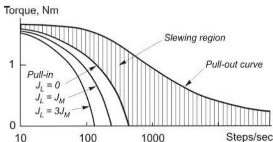
FIG. 10.21 Typical pull-in and pull-out curves showing the effect of load inertia on the pull-in torque.  $J_M$ , motor inertia;  $J_L$ , load inertia.
