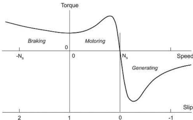
**FIG. 6.16** Torque-speed curve over motoring region (slip between 0 and 1), braking region (slip  $>1$ ) and generating region (negative slip).
