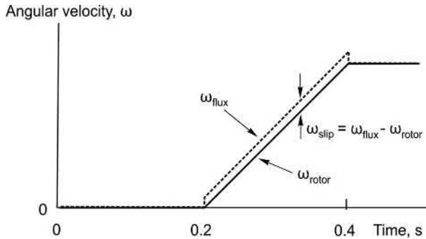
FIG. 8.23 Angular velocity during acceleration.
