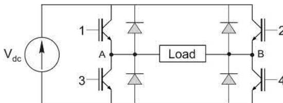
FIG. 2.14 Single-phase inverter.
