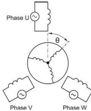
**FIG. 8.5** Coupled-circuit model of 3-phase induction motor.
