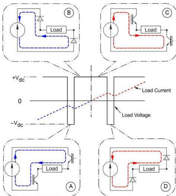
FIG. 2.20 The commutation process in a single-phase bridge.
