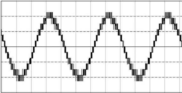
FIG. 2.24 A 13-level inverter voltage waveform.
