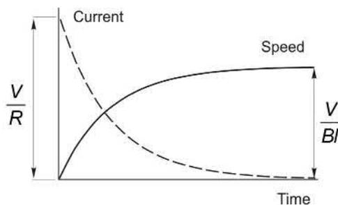
FIG. 1.17 Dynamic (run-up) behaviour of primitive d.c. motor with no mechanical load.
