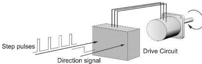
FIG. 10.1 Open-loop position control using a stepping motor.
