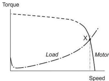
**FIG. 3.8** Steady-state torque-speed curves for motor and load showing location (X) of steady-state operating condition.
