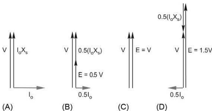
FIG. 9.15 No-load time phasor diagrams showing effect of excitation.
