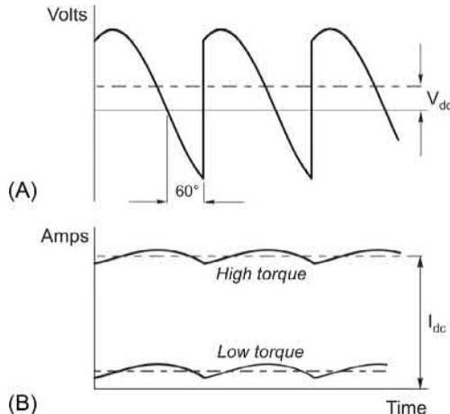
**FIG. 4.3** Armature voltage (A) and armature current (B) waveforms for continuous-current operation of a d.c. motor supplied from a single-phase fully-controlled thyristor converter, with firing angle of 60 degrees.
