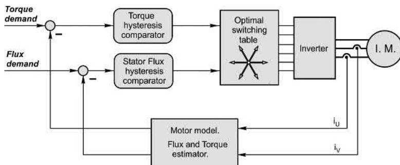
**FIG. 8.24** Block diagram of typical direct torque control scheme.
