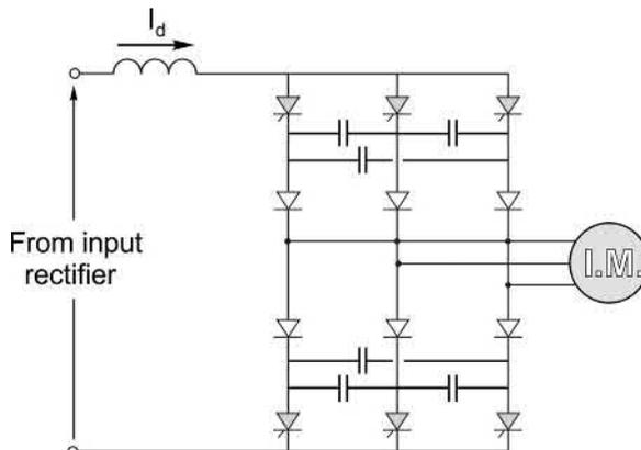
FIG. 7.10 Forced-commutated current-fed induction motor drive (motor converter only shown).
