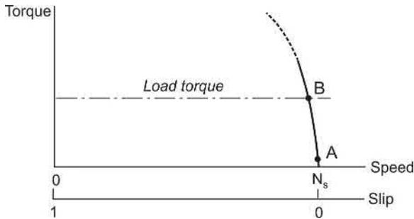
FIG. 5.18 Torque-speed relationship for low values of slip.
