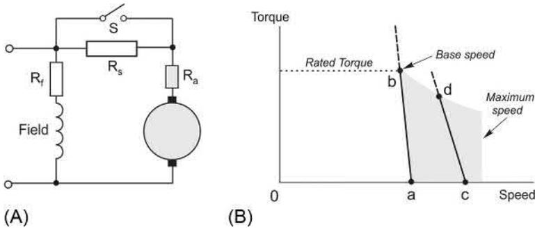
FIG. 3.14 Shunt-connected d.c. motor and steady-state torque-speed curve.
