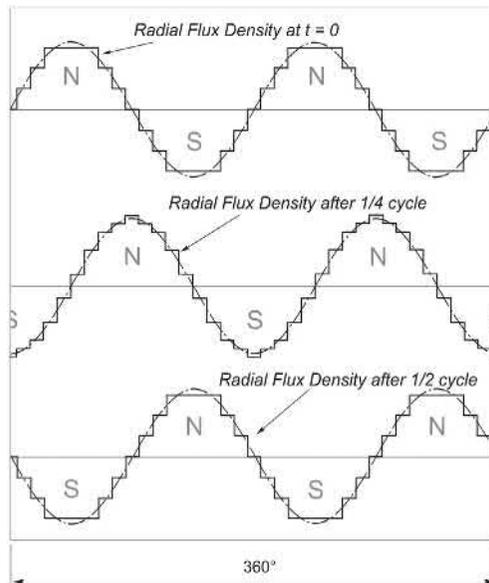
**FIG. 5.8** Resultant air-gap flux density wave produced by a complete three-phase, four-pole winding at three successive instants in time.
