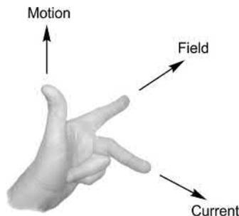
FIG. 1.4 Fleming's Left Hand rule for finding direction of force.
