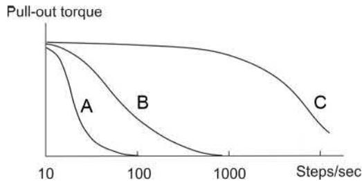
**FIG. 10.18** Typical pull-out torque–speed curves for a given motor with different types of drive circuit. (A) Constant voltage drive; (B) Current-forced drive; (C) chopper drive.
