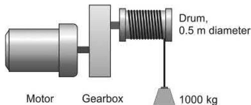
FIG. 11.7 Motor driven hoist—a constant-torque load.
