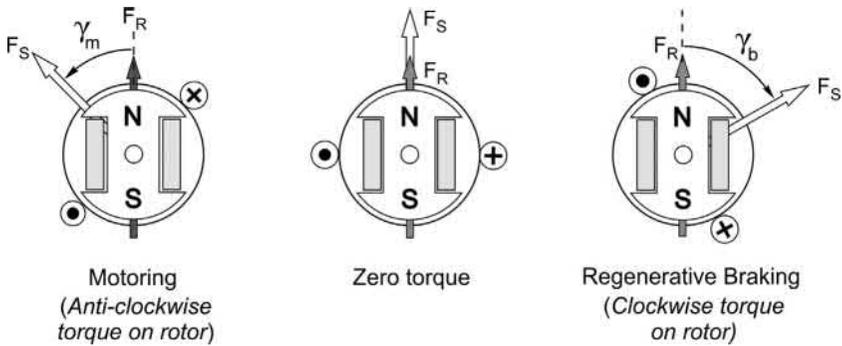
**FIG. 9.23** Synchronous motor showing (left) torque angle ( $\gamma_m$ ) when motoring, and (right) when braking ( $\gamma_b$ ).
