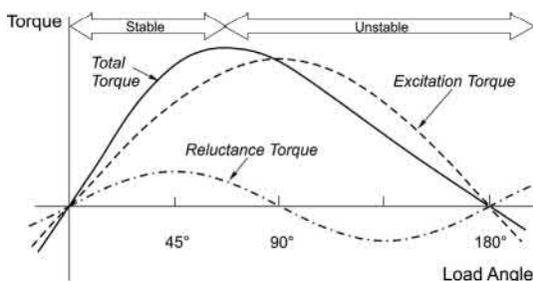
FIG. 9.11 Torque-angle curve for a salient pole excited rotor motor.
