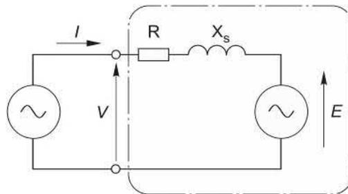
FIG. 9.14 Equivalent circuit for the excited-rotor and PM synchronous machine.
