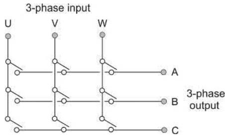
FIG. 2.29 Matrix converter power circuit.
