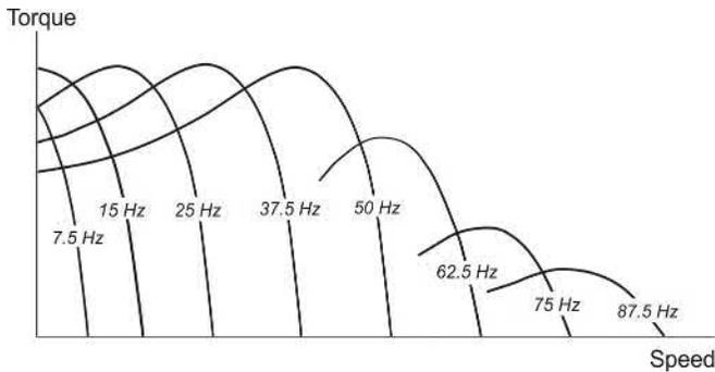
**FIG. 7.4** Typical torque-speed curves for inverter-fed induction motor with constant flux up to base speed (50 Hz) and constant voltage at higher frequencies.
