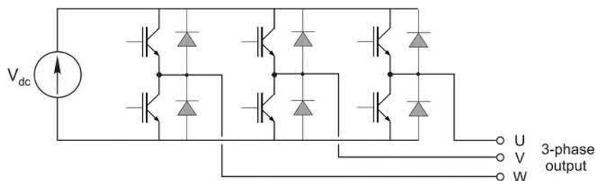
**FIG. 9.28** Three-phase inverter power circuit.
