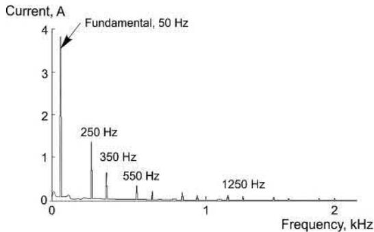
FIG. 7.16 Harmonic spectrum of the improved current waveform shown in Fig. 7.15.
