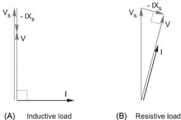
**FIG. 6.2** Phasor diagrams showing the effect of supply-system impedance on the output voltage with (A) inductive load and (B) resistive load.
