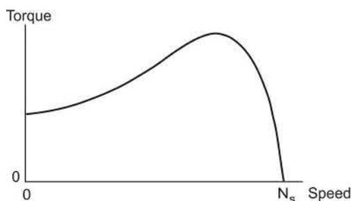
FIG. 5.21 Typical complete torque-speed characteristic for motoring region of cage induction motor.
