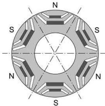
FIG. 9.12 Six-pole PM/Rel motor.
