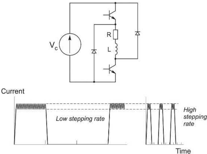
FIG. 10.17 Constant-current chopper drive and typical current waveforms.
