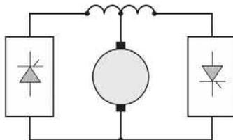
FIG. 4.9 Double-converter reversing drive.
