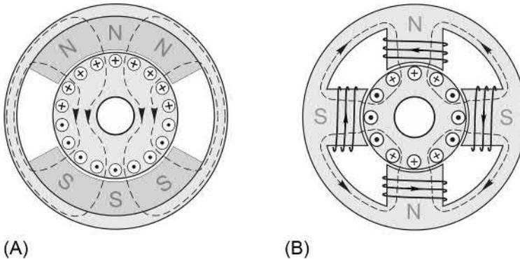
**FIG. 3.2** Excitation (field) systems for d.c. motors (A) two-pole permanent magnet; (B) four-pole wound field.
