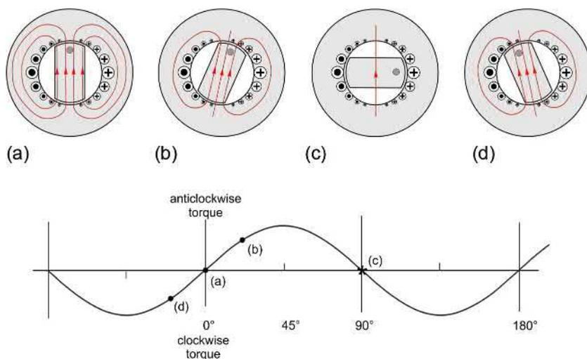
FIG. 9.8 Static torque in a reluctance motor.
