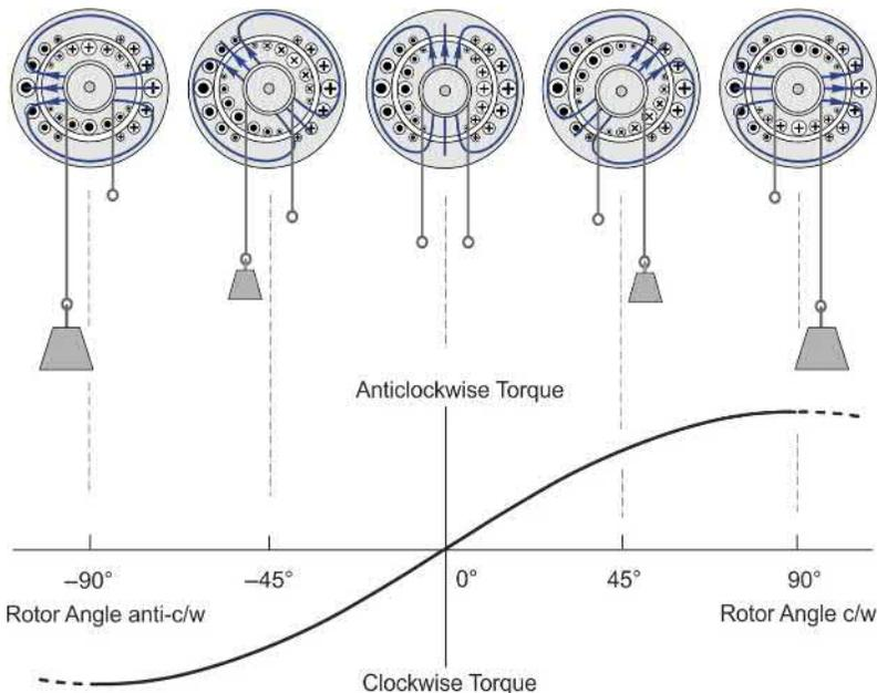
FIG. 9.5 Static torque in an excited rotor motor.
