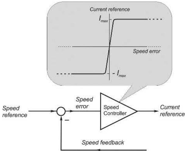
FIG. 4.13 Detail showing characteristic of speed error amplifier.
