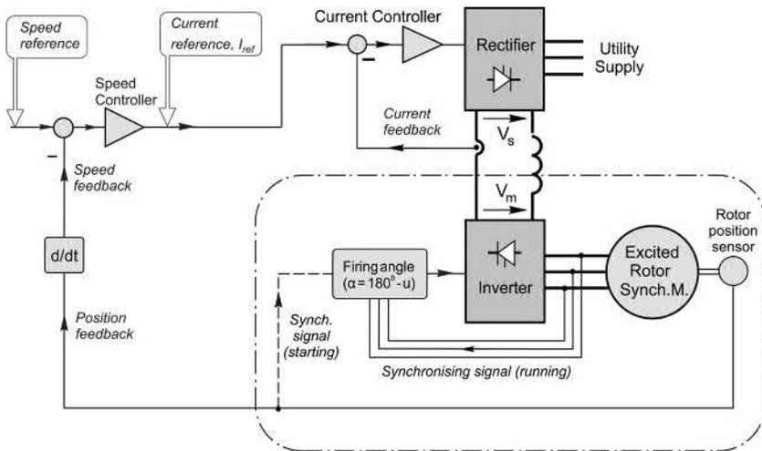
FIG. 9.27 Control scheme for converter fed excited rotor synchronous motor.
