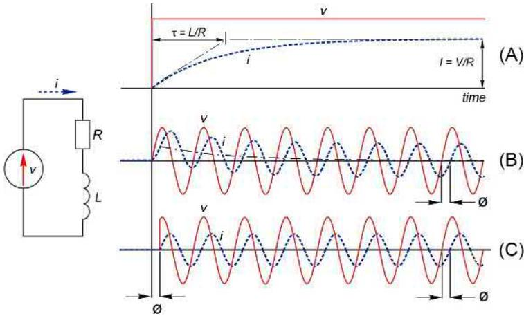
FIG. 8.4 Transition between steady states in series R-L circuit.
