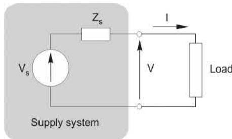
FIG. 6.1 Equivalent circuit of supply system.
