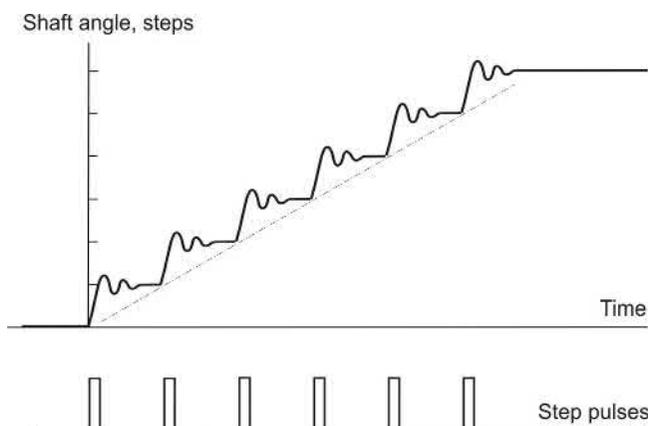
**FIG. 10.2** Typical step response to low-frequency train of step command pulses.
