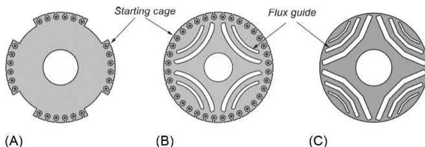
FIG. 9.4 Reluctance motor rotors (4-pole).
