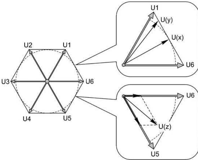
FIG. 8.14 Synthesis of intermediate voltage phasors in vector modulator.
