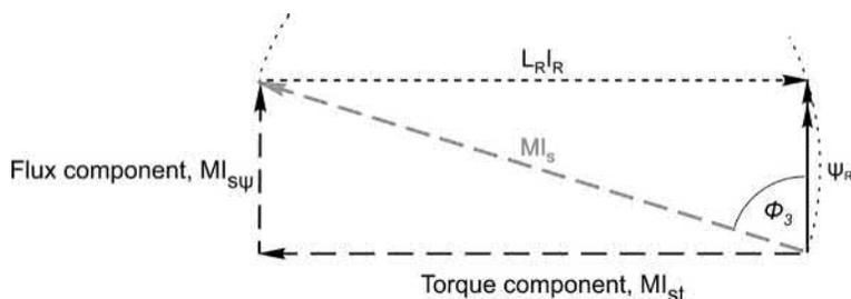
FIG. 8.9 Flux and Torque components of stator current.
