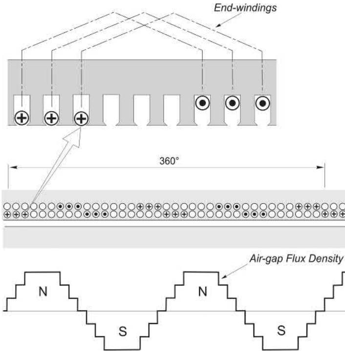
**FIG. 5.5** Developed diagram showing layout of windings in a three-phase, four-pole, two-layer induction motor winding, together with the flux density wave produced by one phase acting alone. The upper detail shows how the coil-sides form upper and lower layers in the slots.
