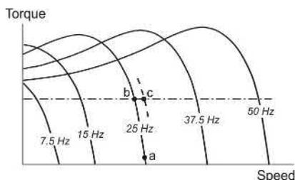
FIG. 7.3 Torque-speed curves for inverter-fed induction motor with constant  $V/f$  ratio.
