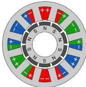
**FIG. 9.39** 10-pole, 3-phase winding in 12 slots.
