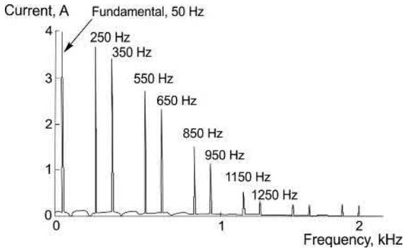
FIG. 7.14 Harmonic spectrum of the current waveform shown in Fig. 7.13.
