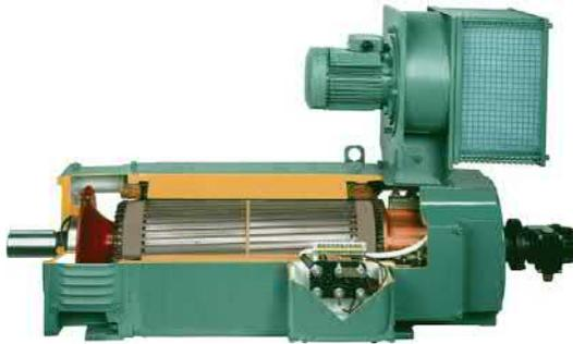
**FIG. 4.2** High performance force-ventilated d.c. motor. The motor is of all-laminated construction and designed for use with a thyristor converter, and has a tachometer mounted at the non-drive end. The small blower motor is an induction machine that runs continuously, thereby allowing the main motor to maintain full torque at low speed without overheating. (*Courtesy of Nidec Leroy Somer.*)
