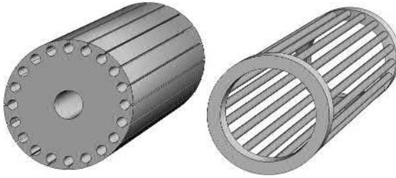
**FIG. 5.11** Cage rotor construction. The stack of pre-punched laminations is shown on the left, with the copper or aluminium rotor bars and end-rings on the right.
