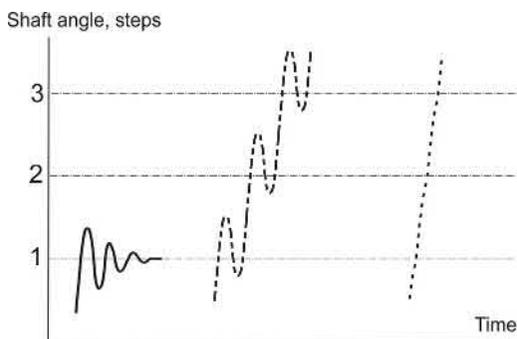
FIG. 10.4 Position-time responses at low, medium and high stepping rates.
