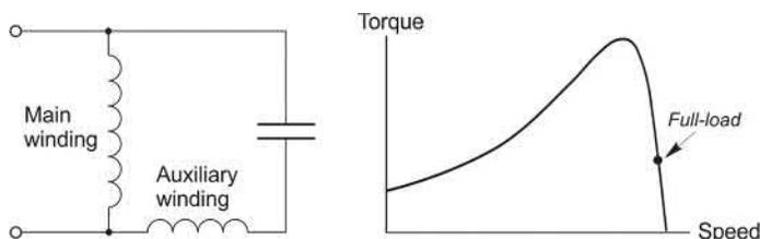
FIG. 6.24 Single-phase capacitor-run induction motor.
