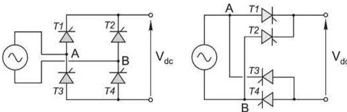
FIG. 2.8 Single-phase 2-pulse (full-wave) fully-controlled rectifier.
