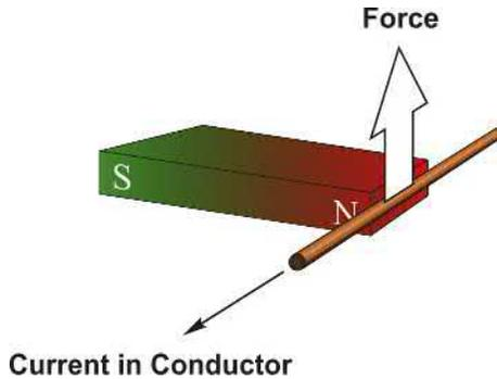
FIG. 1.1 Mechanical force produced on a current-carrying wire in a magnetic field.
