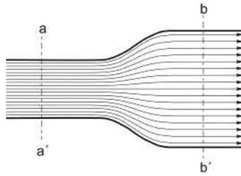
**FIG. 1.3** Magnetic flux lines inside part of an iron magnetic circuit.
