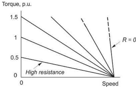
FIG. 6.22 Influence of external rotor resistance ( $R$ ) on torque-speed curve of wound-rotor motor.
