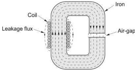
**FIG. 1.8** Flux lines inside low-reluctance magnetic circuit with air-gap.
