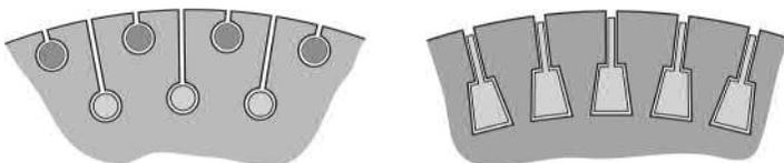
FIG. 6.12 Double cage (left) and deep bar (right) rotors.
