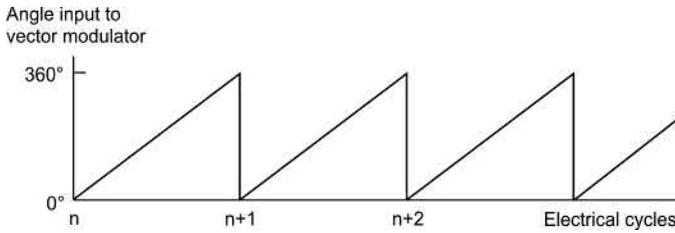
**FIG. 8.15** Angle reference to vector modulator corresponding to constant frequency operation of inverter. (Note that the angle resets to zero at the end of each cycle.)
