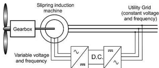
FIG. 6.18 Doubly-fed wound-rotor induction machine for wind power generation.
