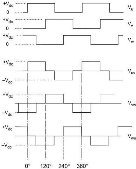
FIG. 2.22 Three-phase square wave output voltage waveforms.
