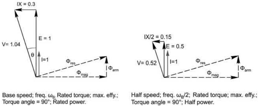
**FIG. 9.21** PM motor phasor diagram—field oriented control. Full rated torque at base speed (left), Full rated torque at half base speed (right).
