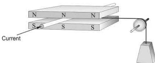
FIG. 1.14 Primitive linear d.c. motor.
