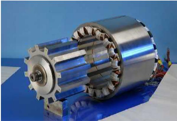
**FIG. 10.22** Switched reluctance motor. The toothed rotor does not require windings or magnets, and is therefore exceptionally robust. (Courtesy of Nidec SR Drives Ltd.)
