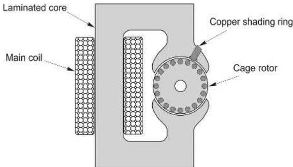
FIG. 6.26 Shaded-pole induction motor.
