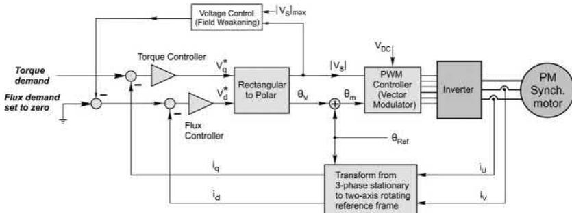
FIG. 9.29 Field oriented control scheme for permanent magnet synchronous motor.
