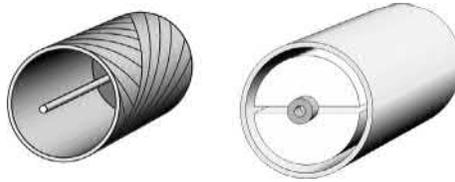
**FIG. 4.15** Ironless rotor d.c. motor. The commutator (not shown) is usually of the disc type.
