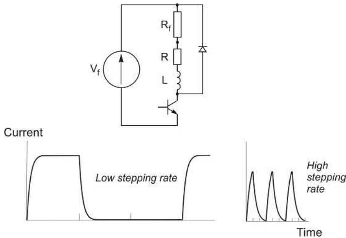
FIG. 10.16 Current-forced ( $L/R$ ) drive and typical current waveforms.
