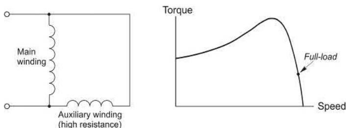
FIG. 6.25 Single-phase split-phase induction motor.
