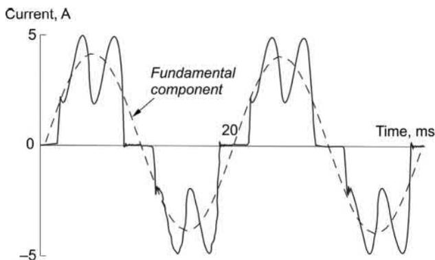
**FIG. 7.15** Utility supply current waveform for a 1.5kW 3-phase drive with d.c. and 2% a.c. inductors.
