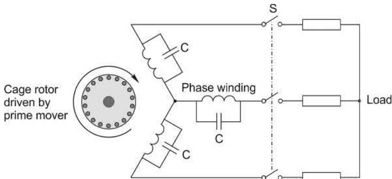
**FIG. 6.17** Self-excited induction generator. The load is connected only after the stator voltage has built up.
