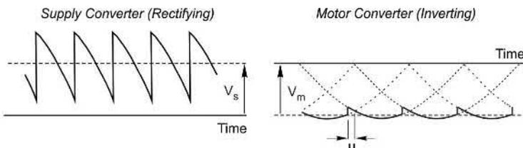
FIG. 9.26 Typical DC link voltages of the current source inverter.
