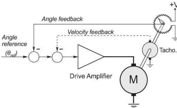
**FIG. 4.16** Closed-loop angular position control using d.c. motor and angle feedback from a servo-type potentiometer.
