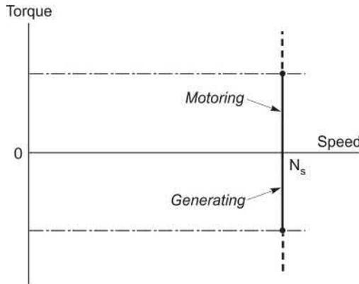
FIG. 9.1 Steady-state torque-speed curve for a synchronous motor supplied at constant frequency.
