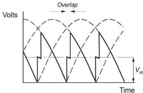
**FIG. 4.6** Distortion of converter output voltage waveform caused by rectifier overlap.
