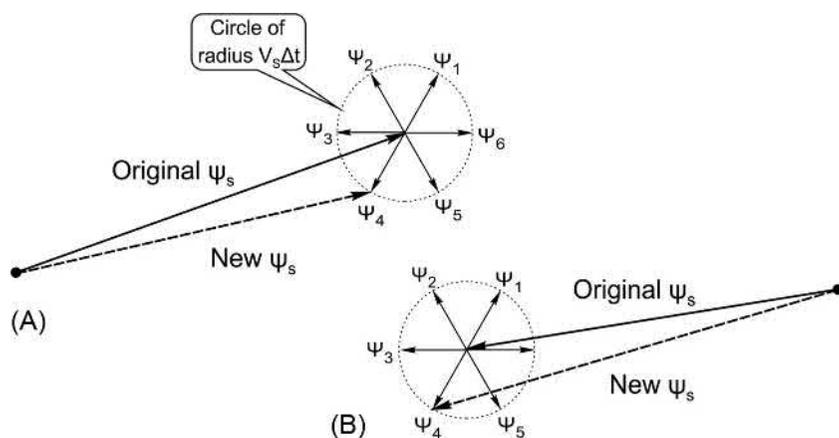
**FIG. 8.25** Space phasor diagram of stator flux linkage showing how the outcome of applying a given volt-second product depends on the original phase angle. In (A) the magnitude is reduced and the phase is retarded, while in (B) the magnitude is increased and the phase is advanced.
