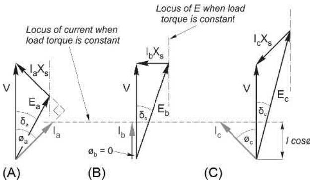
**FIG. 9.16** Phasor diagrams for excited rotor synchronous motor operating with constant load torque, for three different values of rotor (excitation) current.
