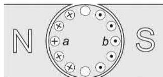
FIG. 3.3 Pattern of rotor (armature) currents in two-pole d.c. motor.
