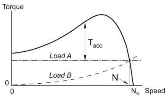
**FIG. 6.5** Typical torque-speed curve showing two different loads which have the same steady running speed (N).
