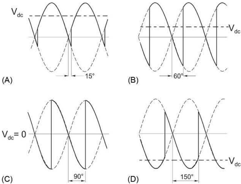
FIG. 2.10 Output voltage waveforms of single-phase fully-controlled rectifier supplying an inductive (motor) load, for various firing angles.
