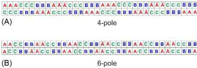
**FIG. 5.7** Developed diagram showing arrangement of three-phase, two-layer windings in a 36-slot stator. A four-pole winding with three slots/pole/phase is shown in (A), and a six-pole winding with two slots/pole/phase is shown in (B).
