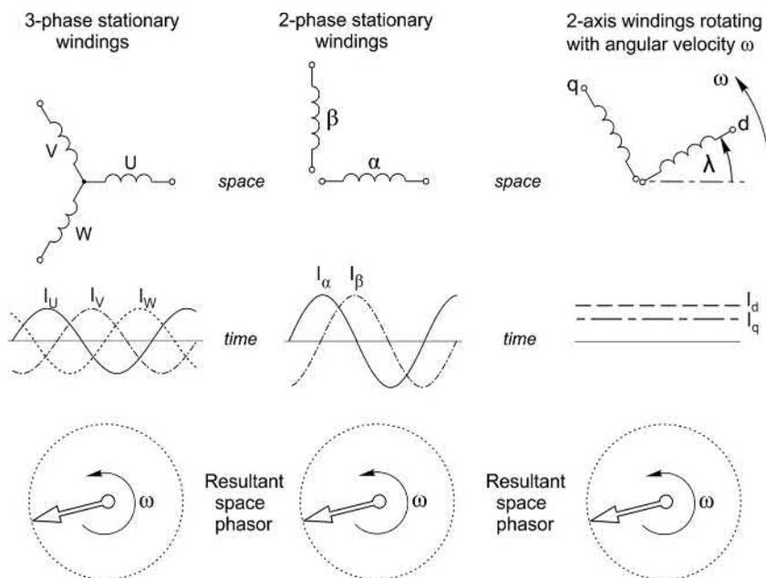
FIG. 8.3 Transformation from 3-phase stationary axis reference frame to two-axis (d-q) rotating reference frame.
