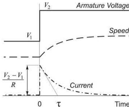
FIG. 3.11 Response of d.c. motor to step increase in armature voltage.
