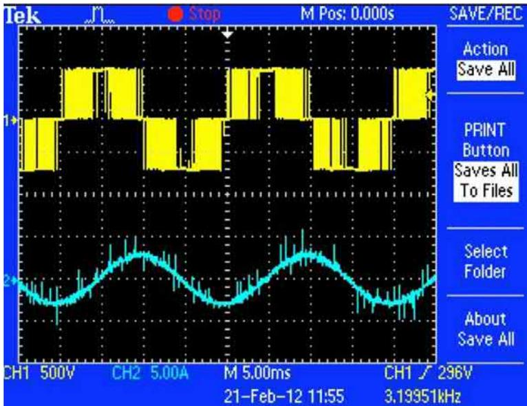
FIG. 7.9 Actual voltage and current waveforms for a star-connected, PWM-fed induction motor. Upper trace—voltage across U and V terminals. Lower trace—U phase motor current.
