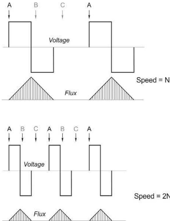
FIG. 10.24 Voltage and flux waveforms for switched-reluctance motor in 'single-pulse' mode.
