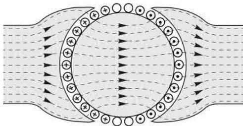
**FIG. 1.12** Current-carrying conductors on rotor, positioned to maximise torque. (The source of the magnetic flux lines (arrowed) is not shown.)
