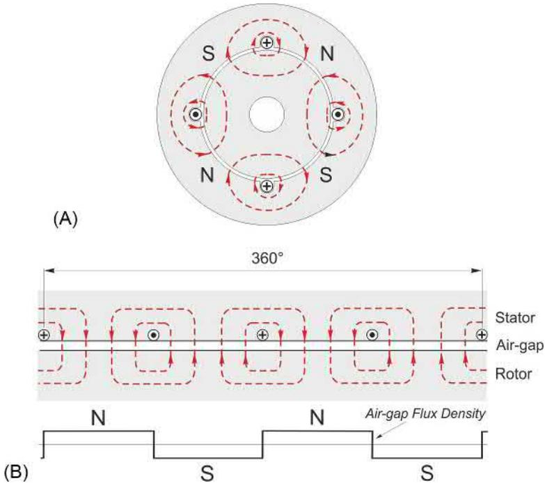
**FIG. 5.3** Arrangement (A) and developed diagram (B) showing elementary four-pole, single-layer stator winding consisting of four conductors spaced by 90 degrees. The ‘go’ side of each coil (shown by the plus symbol) carries current into the paper at the instant shown, while the ‘return’ side (shown by the dot) carries current out of the paper.
