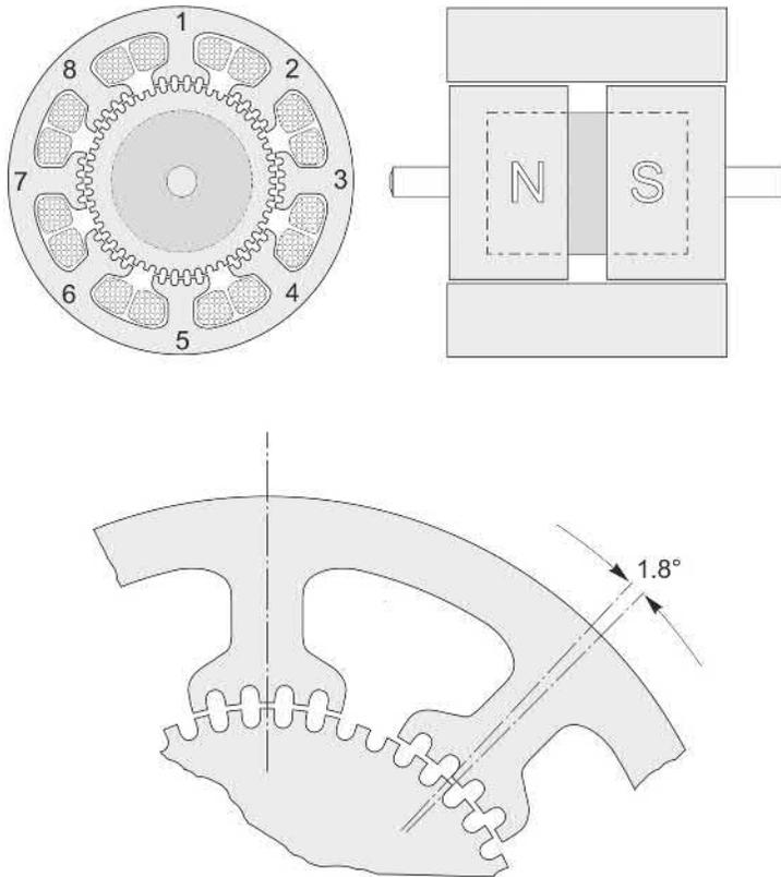
**FIG. 10.6** Hybrid (200 step/rev) stepping motor. The detail shows the rotor and stator tooth alignments, and indicates the step angle of  $1.8^\circ$ .
