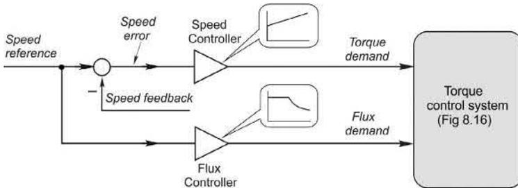
FIG. 8.17 Schematic diagram of closed-loop speed control system.
