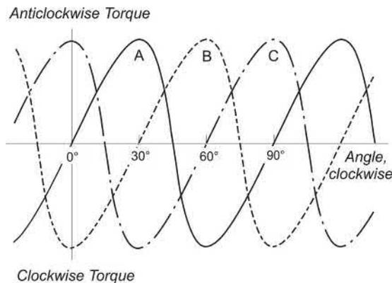
FIG. 10.9 Static torque–displacement curves for  $30^\circ/\text{step}$  variable reluctance stepping motor.
