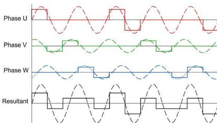
FIG. 9.40 m.m.f. waveform of 10-pole, 3-phase winding in 12 slots.
