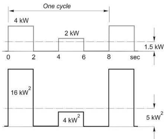
FIG. 11.10 Calculation of r.m.s. power rating for periodically varying load.
