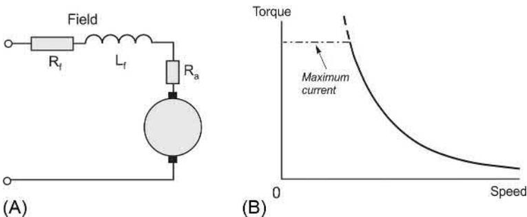
FIG. 3.15 Series-connected d.c. motor and steady-state torque-speed curve.
