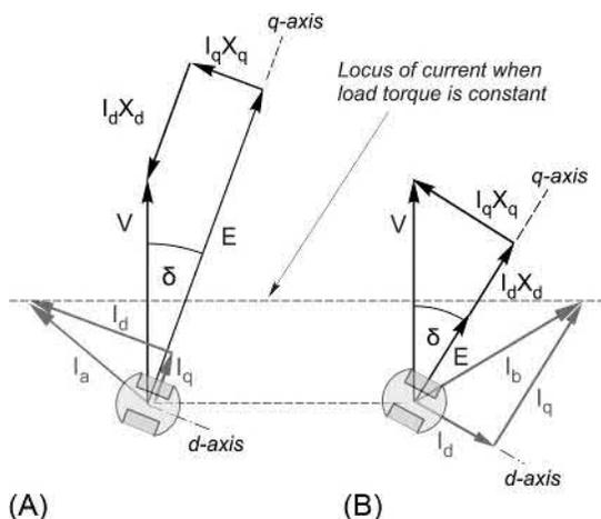
FIG. 9.18 Time phasor diagrams for salient pole excited rotor motor.
