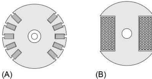
FIG. 9.2 Rotors for synchronous motors. (A) 2-pole cylindrical, with field coils distributed in slots, (B) 2-pole salient pole with concentrated field winding.
