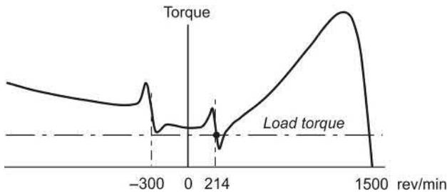
**FIG. 6.8** Torque-speed curve showing the effect of space harmonics, and illustrating the possibility of a motor ‘crawling’ on the 7th harmonic.
