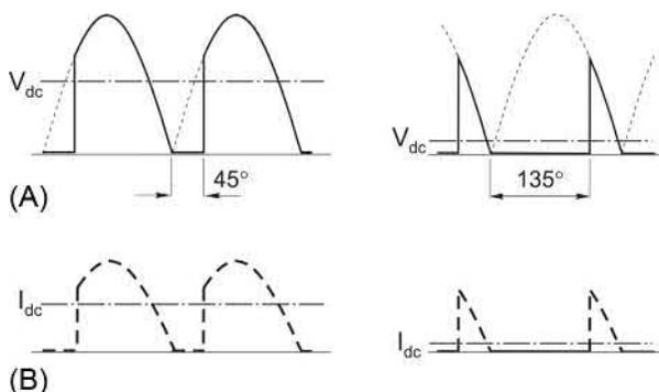
**FIG. 2.9** Output voltage waveform (A) and current (B) of single-phase fully-controlled rectifier with resistive load, for firing angle delays of  $45^\circ$  and  $135^\circ$ .
