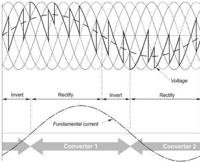
**FIG. 2.28** Typical output voltage waveform for one phase of 6-pulse cycloconverter supplying an inductive (motor) load. The output frequency shown in the figure is one-third of the utility frequency, and the amplitude of the fundamental component of the output voltage (shown by the dotted line) is about 75% of the maximum that could be obtained. The fundamental component of the load current is shown in order to define the modes of operation of the converters.
